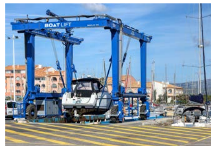
Trave-lift de maintenance © Port Leucate
